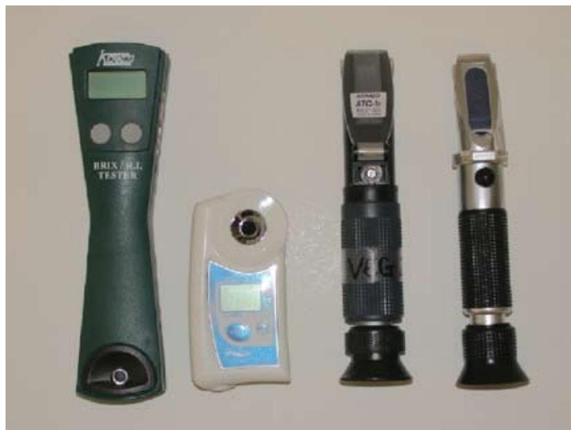
Figure 1. Types of available refractometers. The two on the left are digital and the two on the right are analog.
