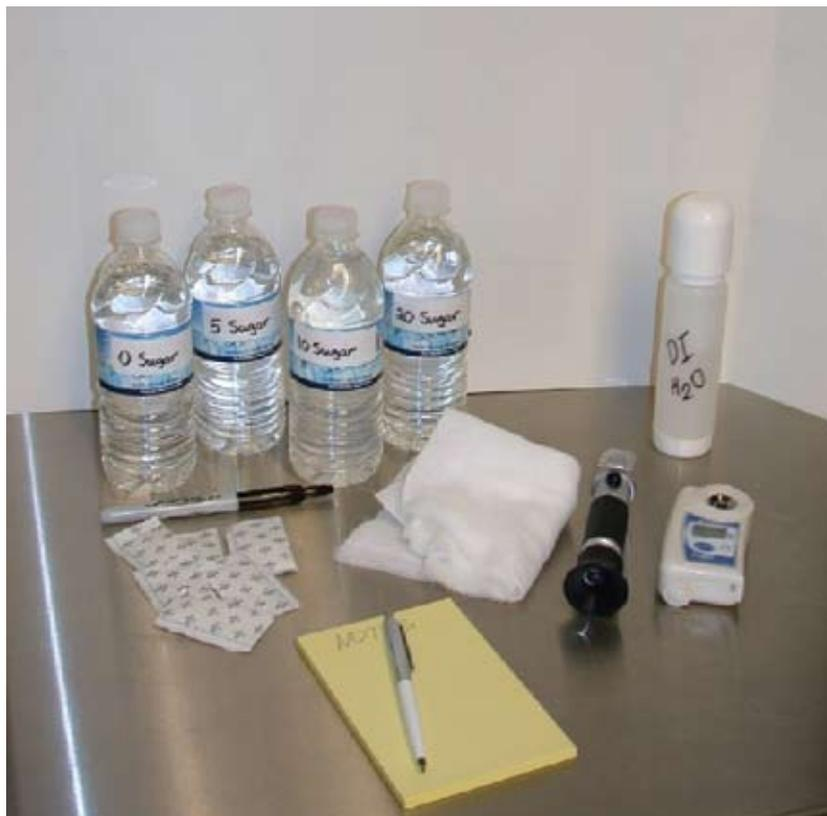
Figure 6. Simple field refractometer calibration test kit.
